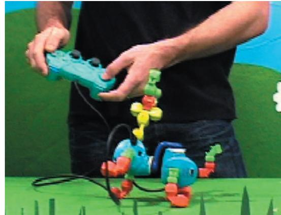
Figure 1: Robo, a modified video game controller, is used to perform a sequence of kinetic recordings with a robotic moose. The moose was designed, built and physically animated using the Topobo system.
